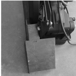
9.6 The iron filings collection box is hookable on the machine, which is designed to gather cutting scraps and facilitate tidying up.
